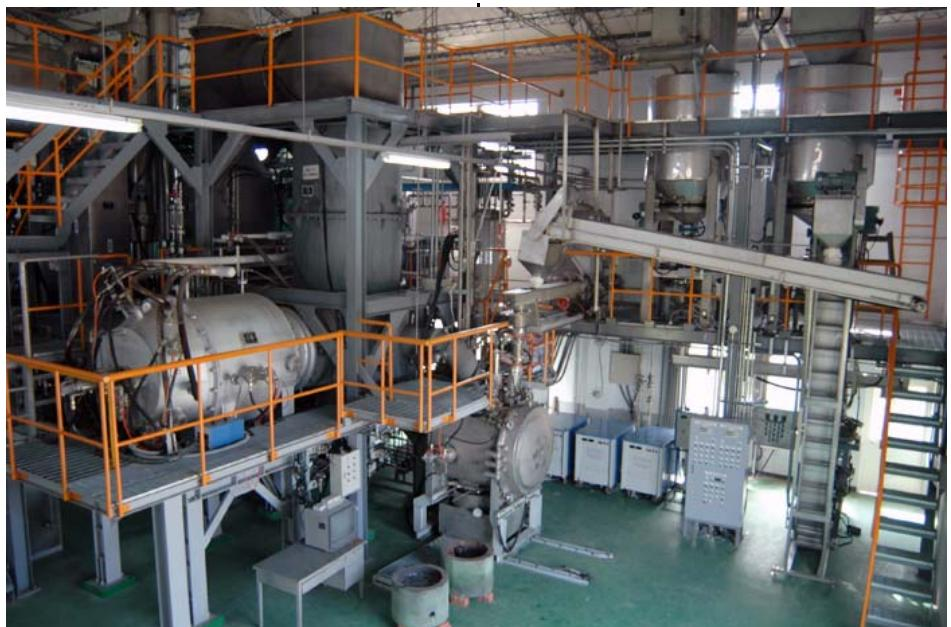
Plasma Melting and Gasification System
